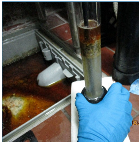
FIGURE 26. ENVIRONMENTAL INSPECTOR TAKING A CORE SAMPLE FROM A GREASE TRAP
