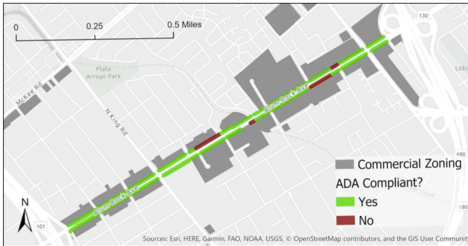
Figure 20: ADA sidewalk Compliance on Alum Rock Avenue
