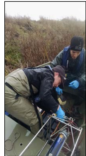
ESD staff maintaining the sonde deployed at Alviso Slough
