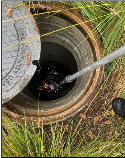
Wet weather PCBs/mercury sampling station at a manhole in the San Thomas Aquino Creek watershed
