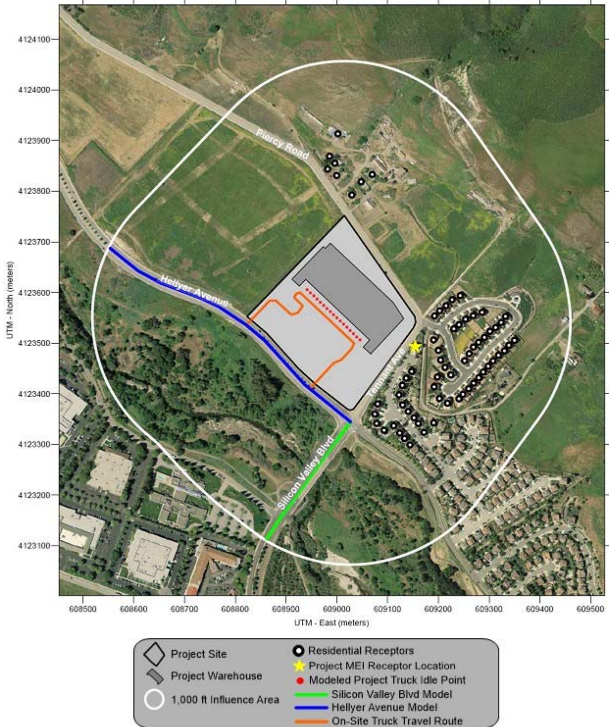
Figure 2. Locations of Project Site, Off-Site Sensitive Receptors, Road Segments Evaluated, and Maximum TAC Impact (Project MEI)
