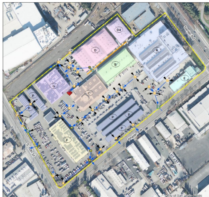
Figure 3: Location of storm drain inlets
