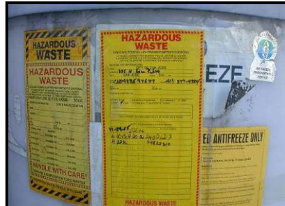
Figure 8: Hazardous waste identified with accumulation dates
