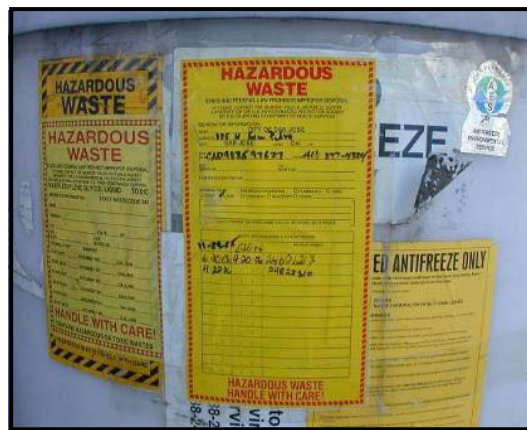
Figure 5: Hazardous waste identified with accumulation start dates.
