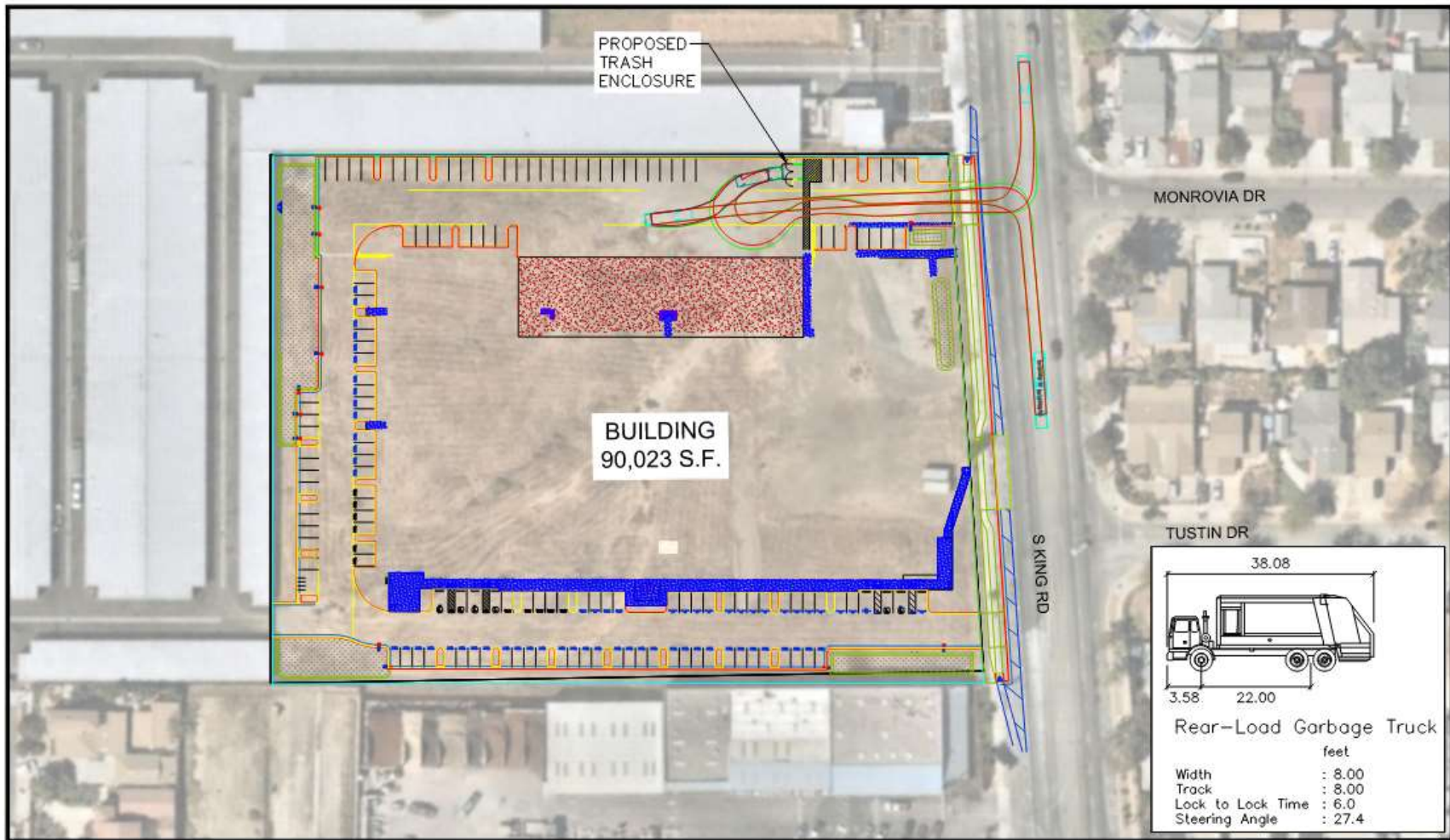
Figure 15: Garbage Truck Access
