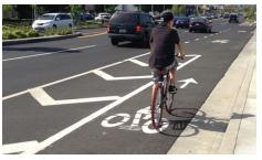
Buffered bike facilities that provide increased separation from motor vehicles with pavement markings
