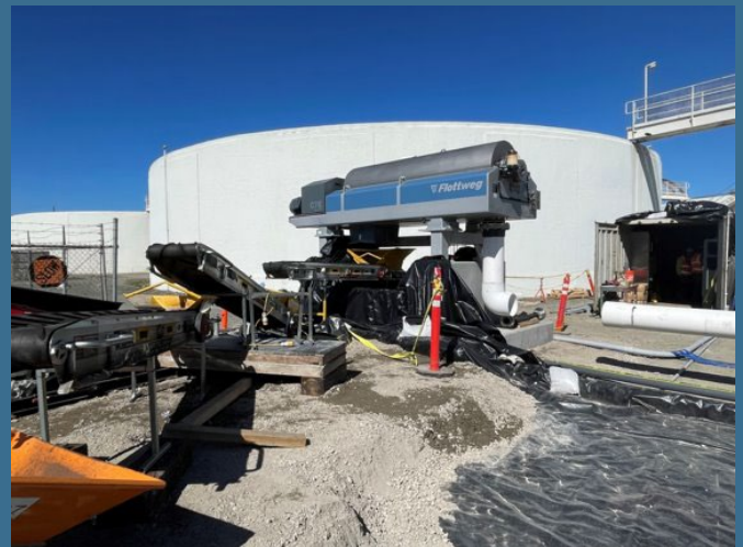
Centrifuge and conveyors setup for confirmation testing
