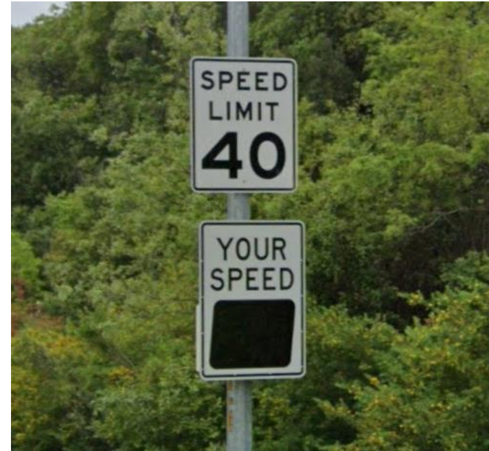
Speed Radar Signs
