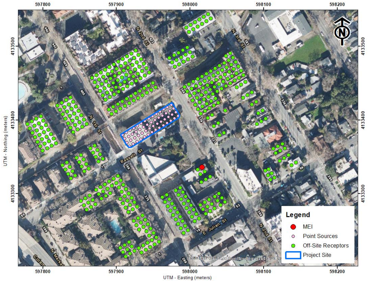
Figure 1. Locations of Project Construction Site, Point Sources, Off-Site Sensitive Receptors, and Maximum TAC Impacts (MEI)
