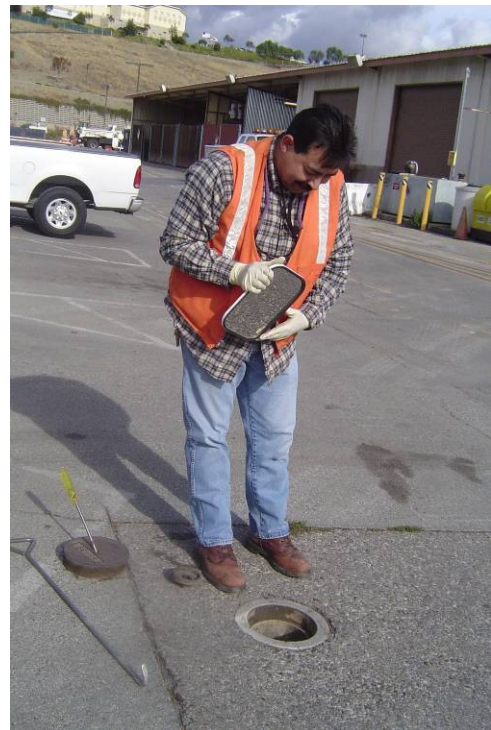
Watershed Enforcement Inspector dye testing for illicit connections
