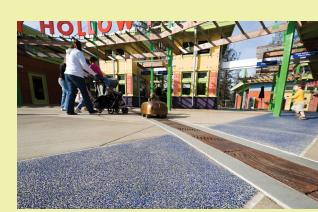
Salvaged blue and green glass bottles were crushed to create the pavement design at the entrance gate.
