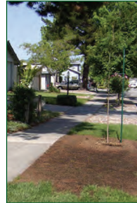
A minimum of two feet should be kept free of turf at the base of a tree
