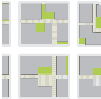
Break up dense development with a network of small, informal-use open spaces.
