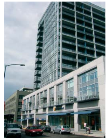
If taller buildings are not oriented parallel to the street, a shorter building can form the street wall.
