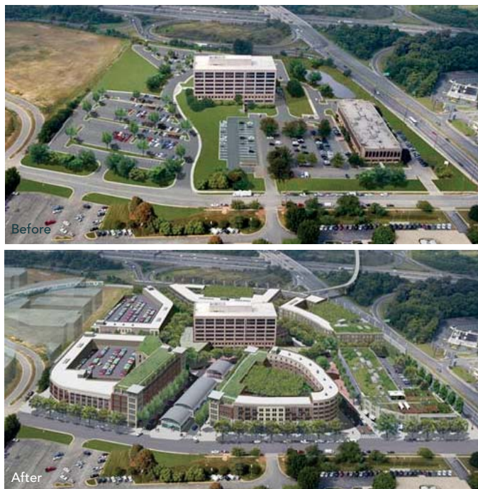
These images show a before-and-after scenario of good site infill, where existing buildings are kept, new street-facing buildings are built on existing parking lots, and surface parking is replaced with parking structures interior to the block.
