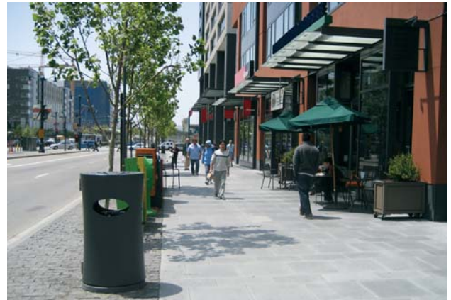
A widened urban sidewalk as envisioned along North First Street includes different zones for sitting, walking, and amenities.
