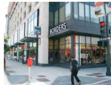
The first two floors should respond to the pedestrian scale with clear glazing, columns, awnings, recesses, and signage.
