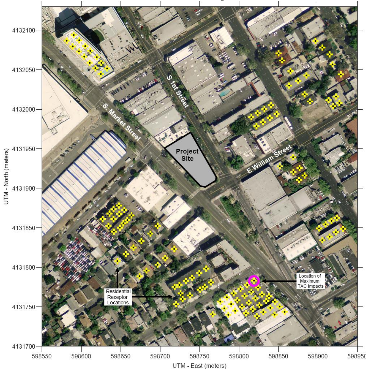
Figure 2. Project Construction Site, Locations of Off-Site Sensitive Receptors and Maximum TAC Impacts
