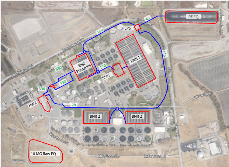
Flow equalization will provide the peak wet-weather flow management for the treatment train.
