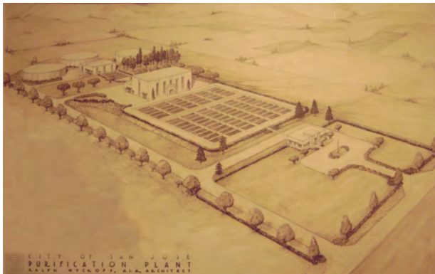
The original Plant was operated by eight workers and consisted of just primary treatment, three digesters, and a small pump and engine building.
