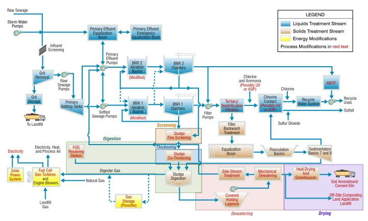
The solids treatment processes are comprised of sludge fine screening, sludge thickening, digestion, dewatering, and drying.
