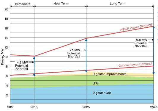
Plant-generated power is close to matching the estimated power demand for critical operation. However, a significant shortfall exists for meeting the power demand for full operation.
