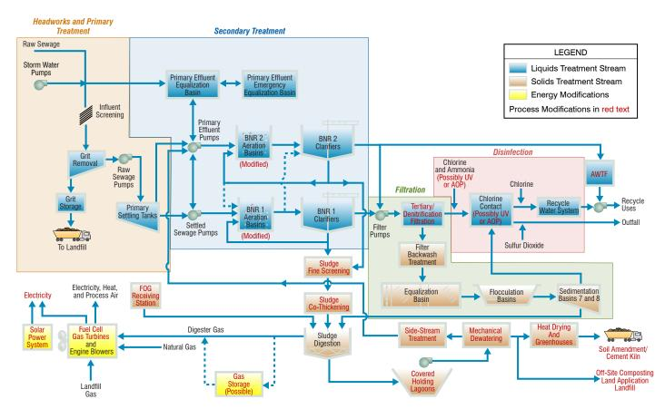
The liquids treatment processes are comprised of headworks and primary treatment, secondary treatment, filtration and disinfection.
