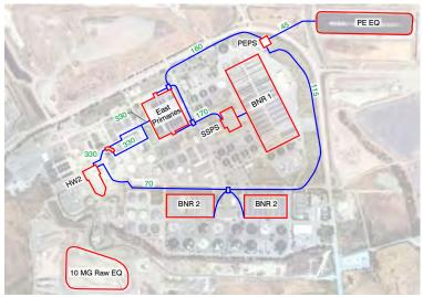
Flow equalization will provide the peak wet-weather flow management for the treatment train.
