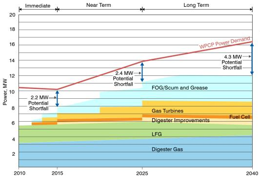
The power shortfall can be offset partially through the incorporation of various new technologies at the Plant, and the introduction of outside, high-energy feedstocks.
