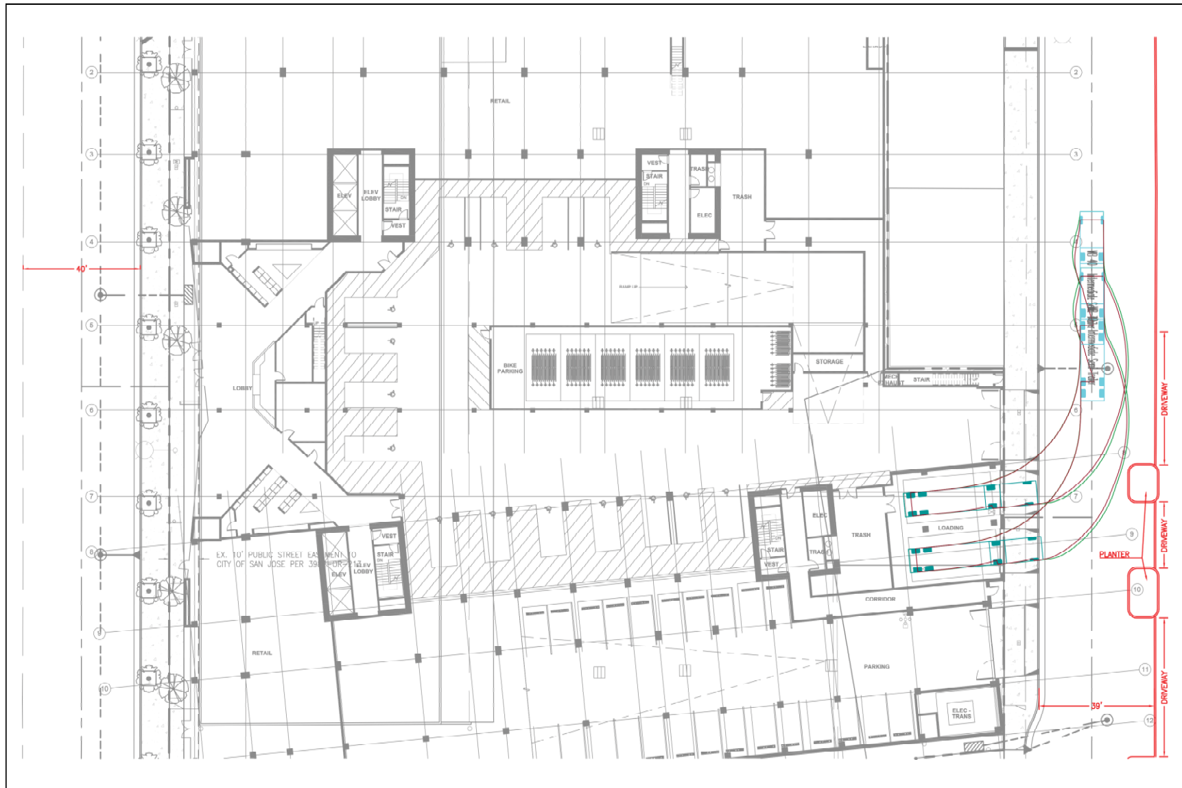
Figure 7 Truck Turning Paths (WB 40 Truck)
