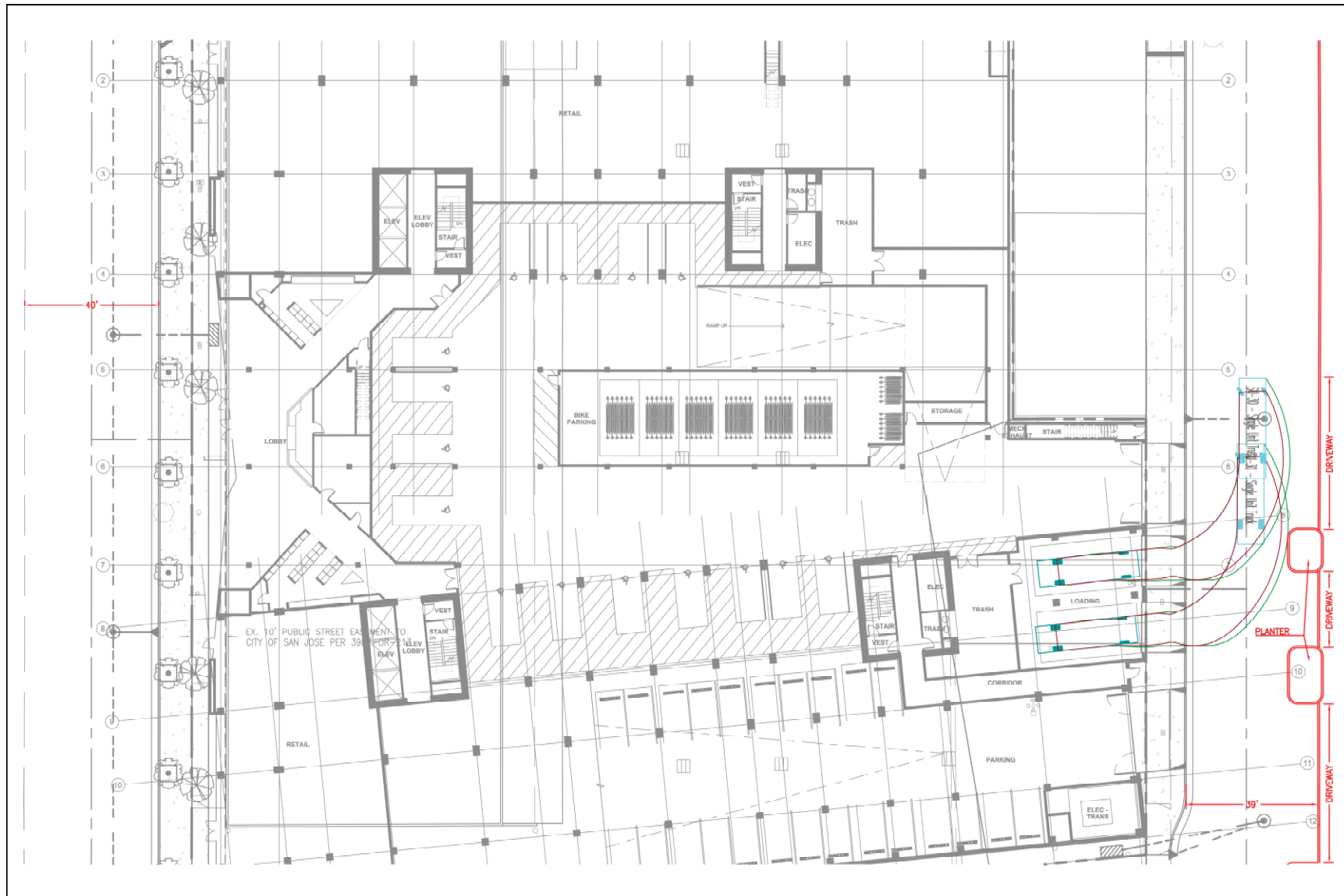
Figure 6 Truck Turning Paths (WB 30 Truck)
