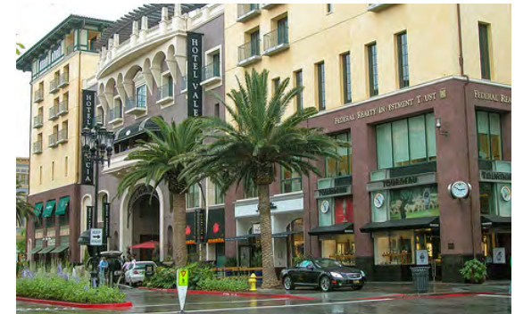
▶ Ground floor retail, differentiated from the upper floors by a change in color, materials, and recessed storefronts that are separated from each other.
