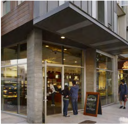
Ground floor retail with large windows and few mullions create better a connection between the interior space and the sidewalk encouraging pedestrians to stop, look and go inside.
