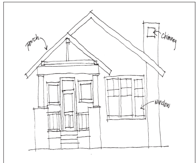
Inappropriate drawing: the scale and character are not clearly conveyed, nor are there any dimensions.
