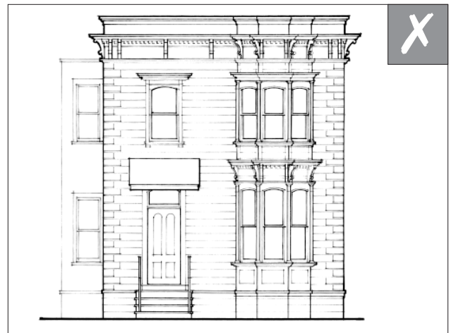
Existing Condition: Italianate style house with the original porch removed.
