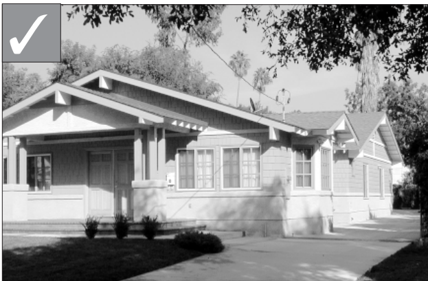
Subdividing a larger building mass into smaller “modules” that are similar in size to buildings seen traditionally is encouraged. This new house is divided into modules, which is appropriate. (Pasadena, CA)
