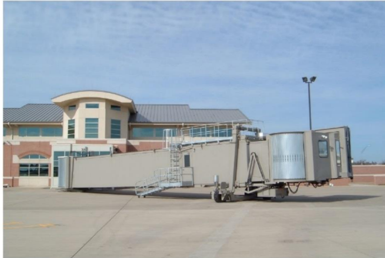
Photo 1: Example of a Radial Boarding Bridge
