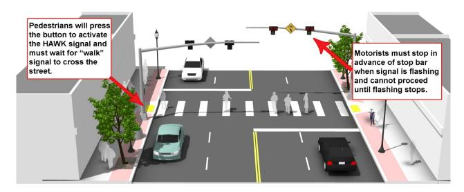
A High Intensity Activated Crosswalk (HAWK) signal is a traffic control device used to stop road traffic and allow for protected crossing of pedestrians and cyclists when needed.
