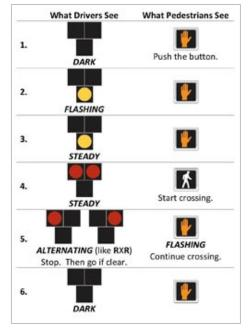
crosswalk. When vehicles have the right-of-way, the pedestrian signal heads go to steady "Don't walk". Then, the HAWK beacons go dark and the pedestrian signal heads remain in the "Don't walk" mode until the HAWK signal is activated by another pedestrian.
