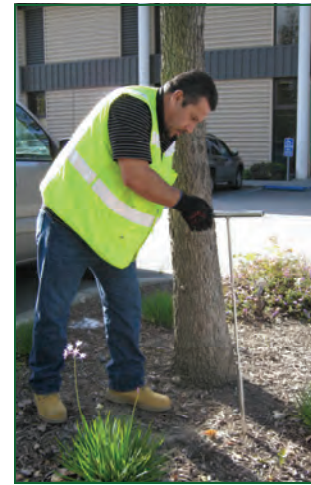
Using a 1" diameter soil probe to check for soil moisture.
