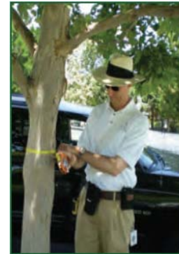
Measuring the DBH of a tree
