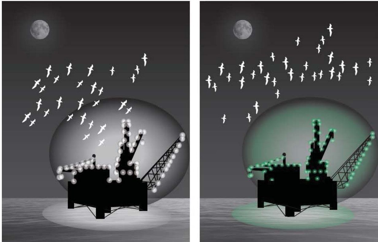
Figure 19. Green lights have been investigated for use on offshore structures and shown to be less attractive to birds.
