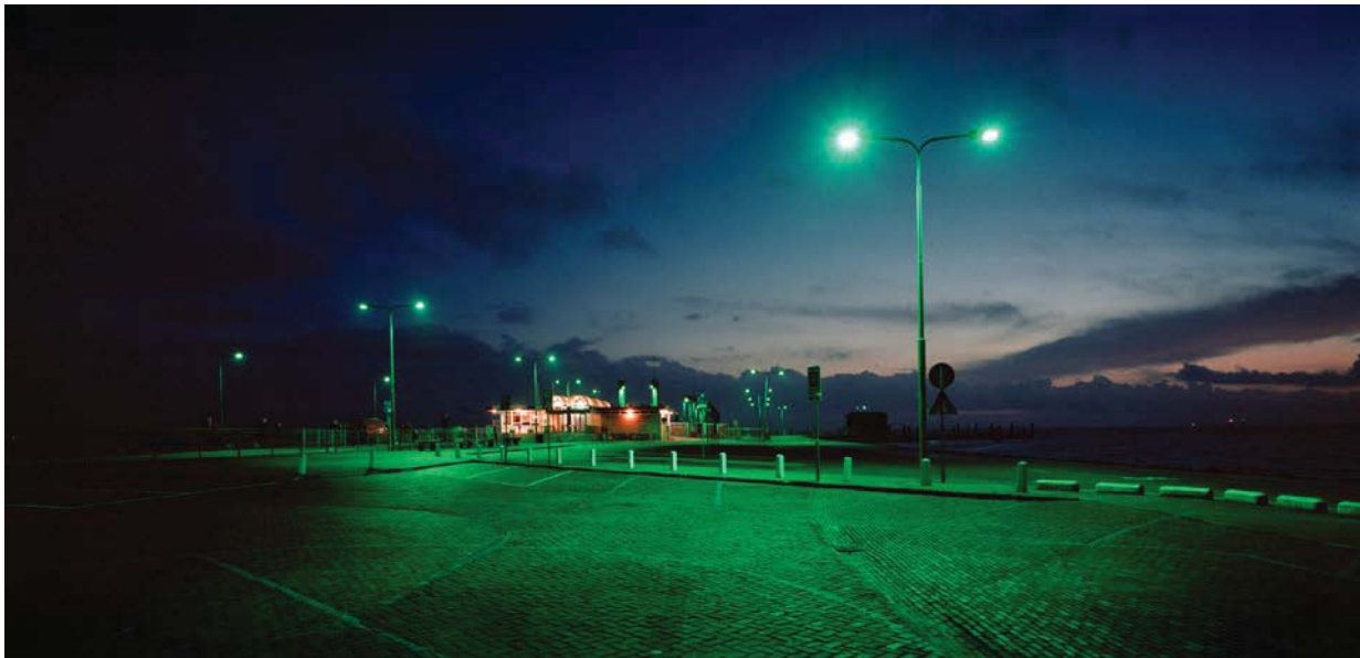
Figure 18. Green lighting designed to minimize attraction of birds developed by Philips. Shell is using these lights on an oil platform in Alaska and Philips is adding the lights to its regular catalog. Photograph courtesy of Joop Marquenie.
