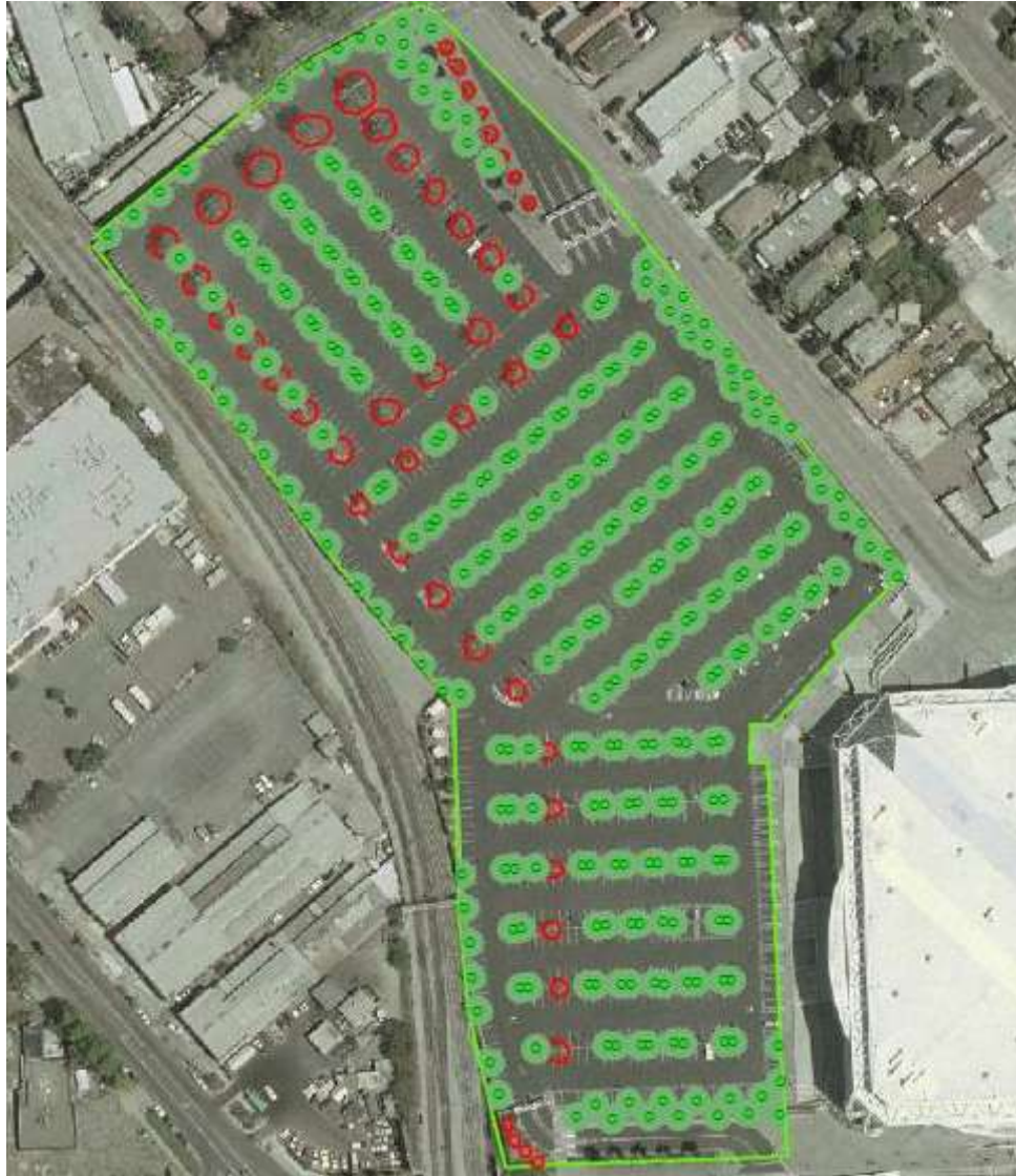
Figure 18. Appendix I Medium tree design for the parking lot PTPS demonstration. PTPS locations (light green dots), their 30ft-diameter crowns (dark green circles), and existing canopy (delineated in red) are shown.
