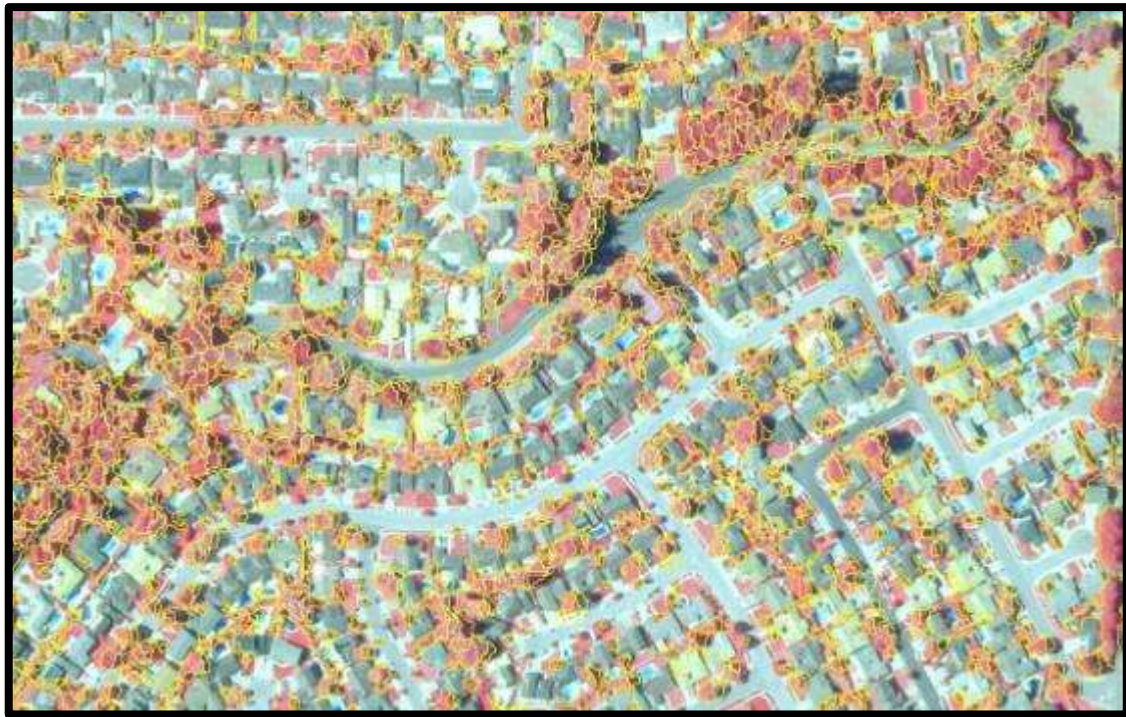
Figure 8. Segmented tree-canopy objects generated to facilitate manual review and correction.
