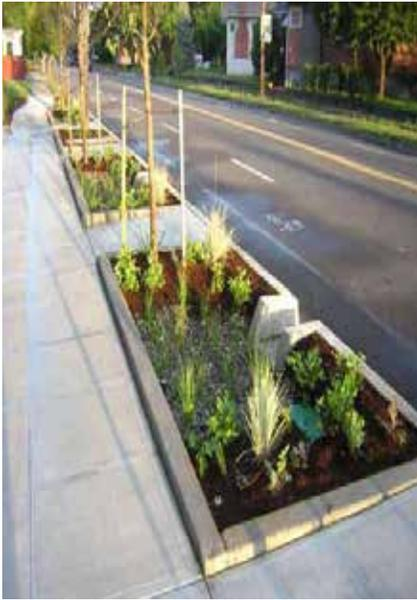
Rain gardens and infiltration planters can be used to mitigate stormwater runoff.
