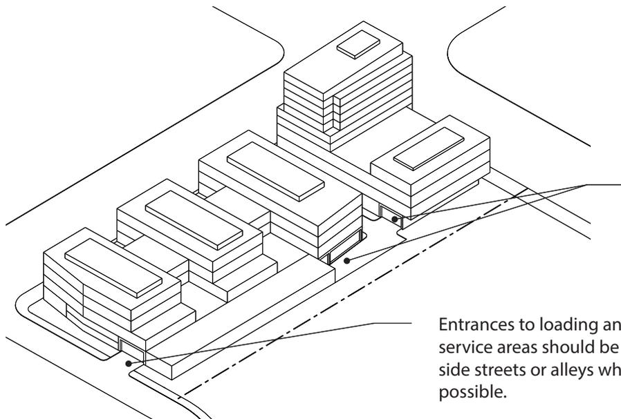
Loading and service areas shall be located at the rear of a property, in structures, or in the interior of blocks.
