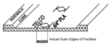
d. **Corridor Marking:** Used to mark multiple facilities of the same type (e.g., electric), bundled or intertwined in the
