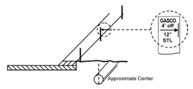
4. An operator's identifier (name, abbreviation, or initials) is placed at the beginning and at the end of the proposed work. In addition, subsequent operators using the same color mark their company identifier at all points where their facil-
