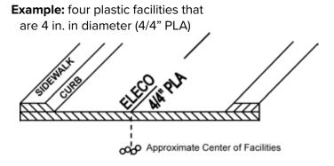
c. **Conduit Marking:** Used for any locatable facility being carried inside conduits or ducts. The marks indicating the outer extremities denote the actual located edges of the facilities being represented.
