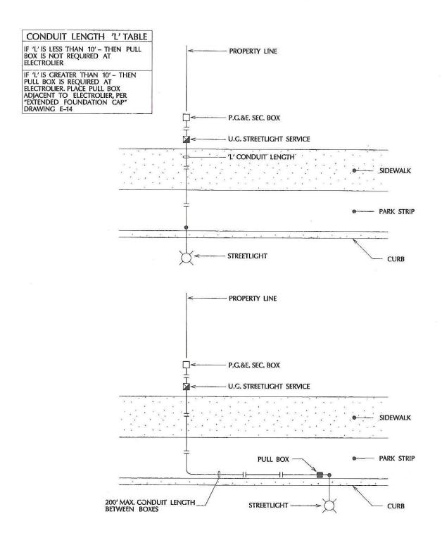
NOTE: SEE DRAWINGS E-33, E-34, E-35, AND E-36 FOR UNDERGROUND SERVICE REQUIREMENTS.
