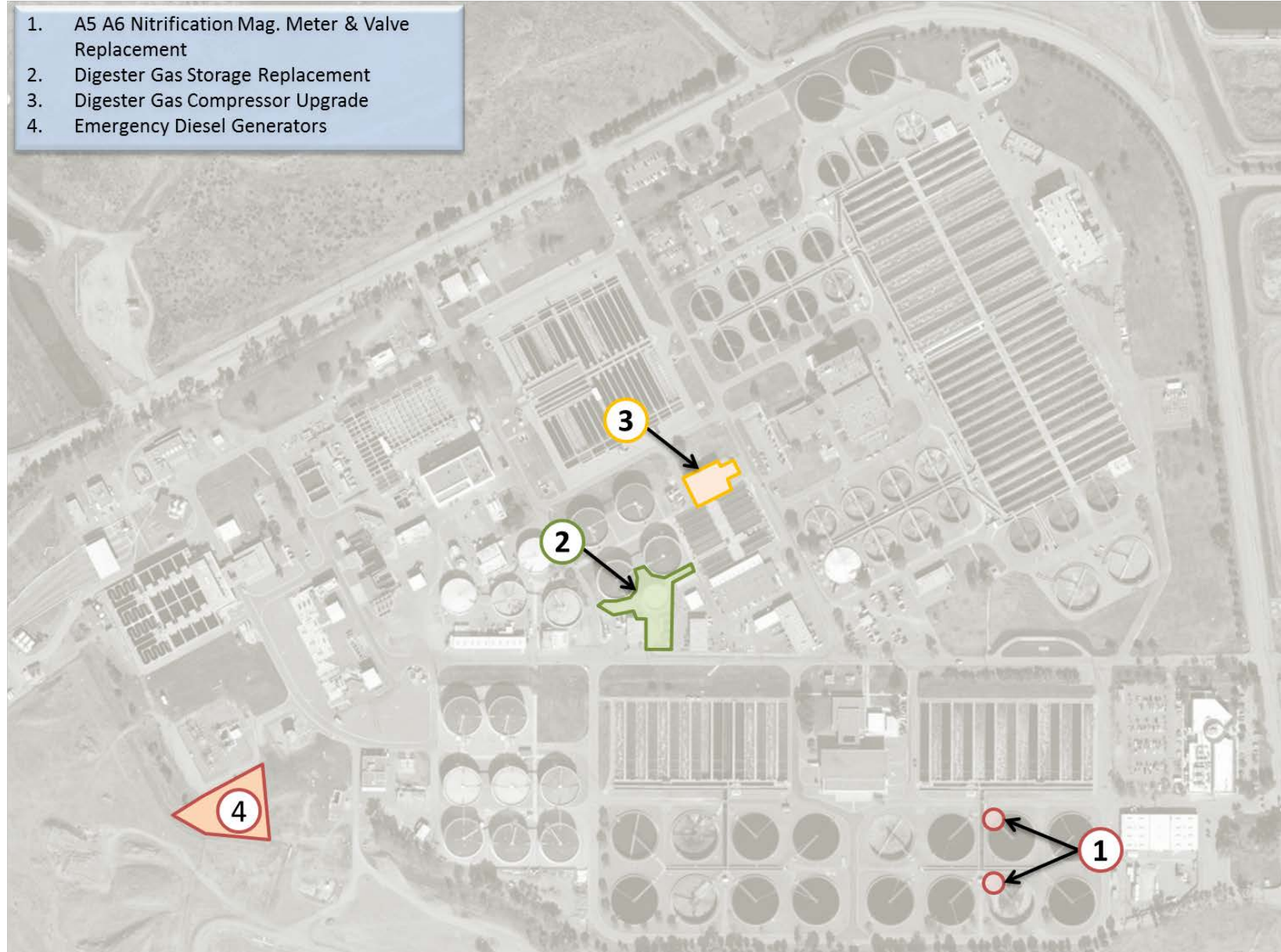
Figure 5—Active Construction Projects
