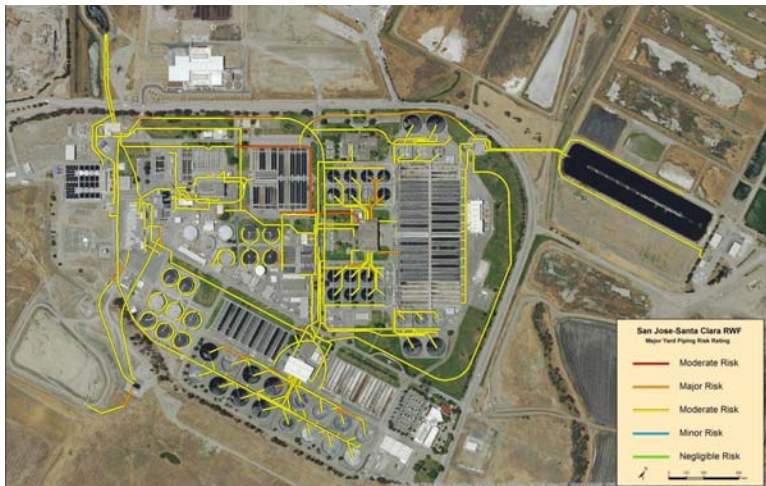
Figure 1: RWF process piping highlighted by risk rating
