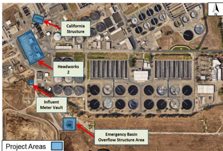
Figure 3: RWF facilities that will be impacted by the Headworks Critical Improvements Project
