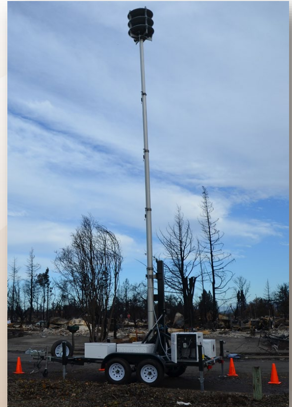
Long-Range Acoustical Device (L-RAD)
