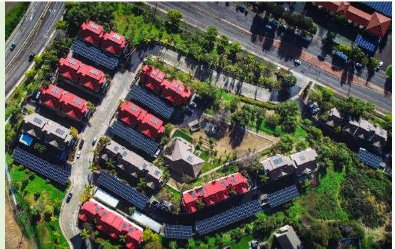
Illustrated Design Principle: In this retrofit scenario there were no additional costs to transition to electric stoves and heat pumps, and the project was able make a profit off the 100% solar offset array.
