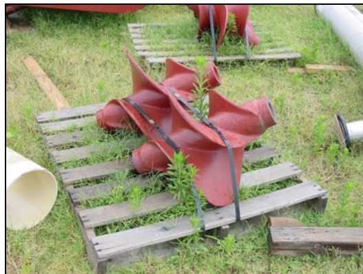
Figure 4-5. Mechanical draft tube mixer impellers
