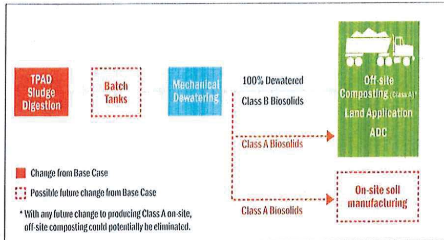
Figure 4: Alternative 3 – Thermophilic Digestion with Future Batch Tanks
