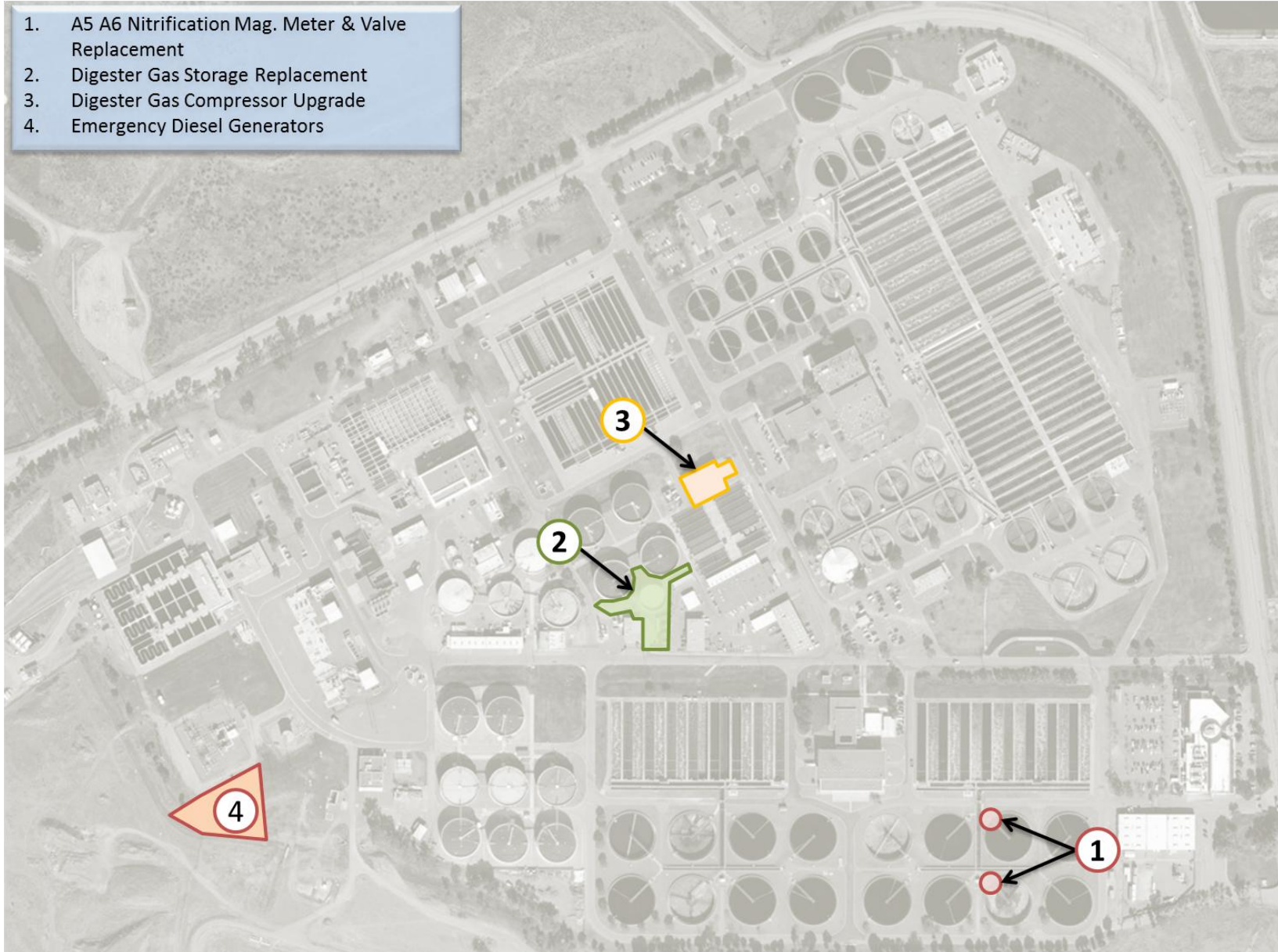
Figure 6—Active Construction Projects
