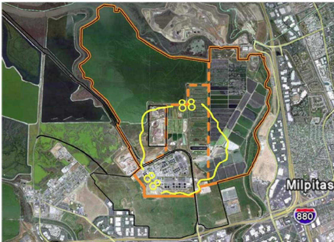
Figure 1—The yellow line shows odor impacts of all potential RWF odor sources within the odor fence line (solid orange line) after Phase 1 odor control implementation.
