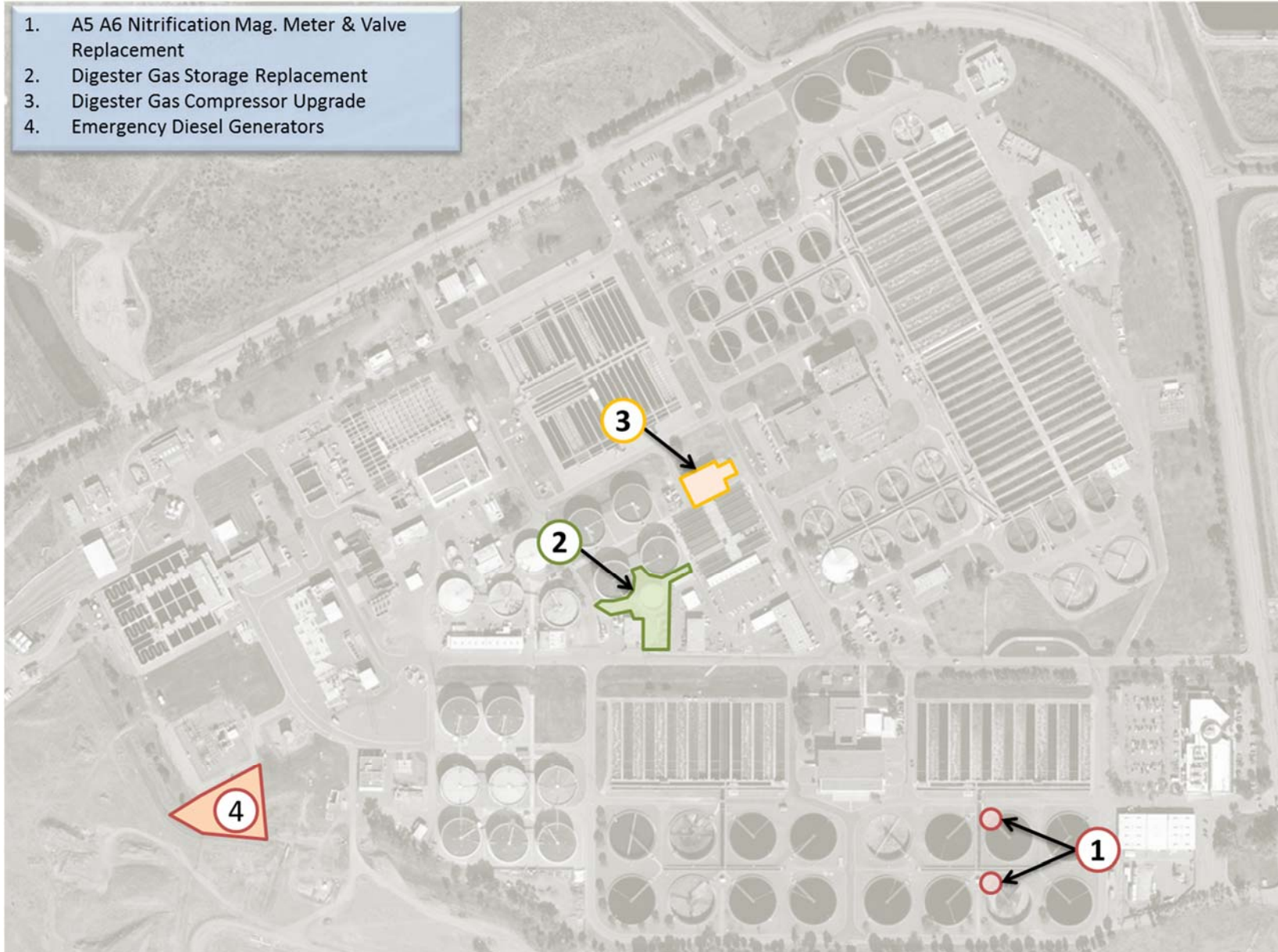
Figure 5 - Active Construction Projects
