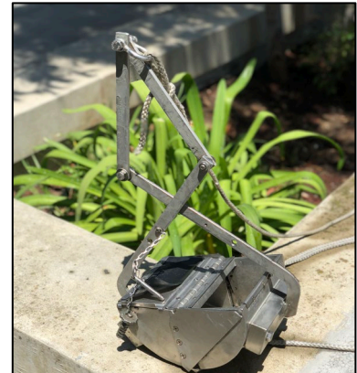
Ponar sediment grab used to collect benthic samples.
