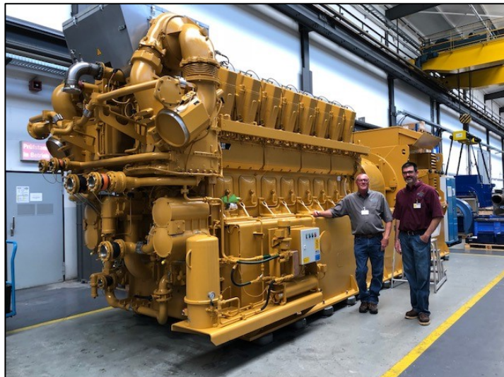
Energy and Automation Division Manager, Ron Nickels, and Power and Air Supervisor Phil Hamilton next to a new 3.5MW CG260-16 engine generator.
