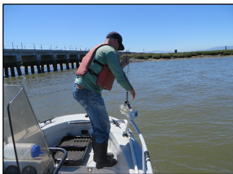
Ryan Mayfield using a Van Dorn sampler to collect a phytoplankton.
