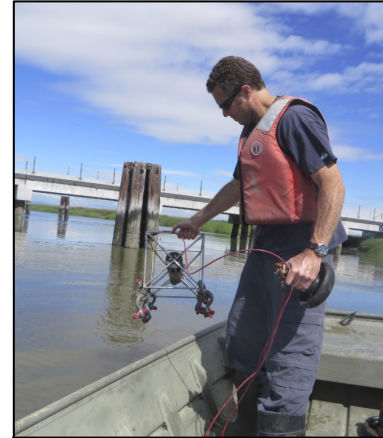
Bryan Frueh, deploying the continuous monitoring sonde.
