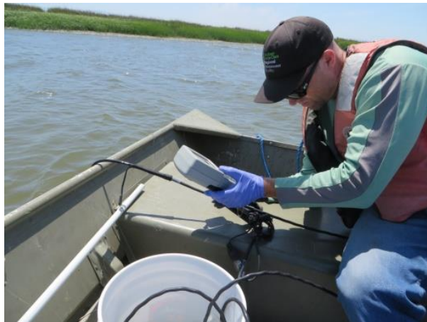
Figure 14. Environmental Services Specialist, Ryan Mayfield, records water quality measurements using a multi-probe YSI
