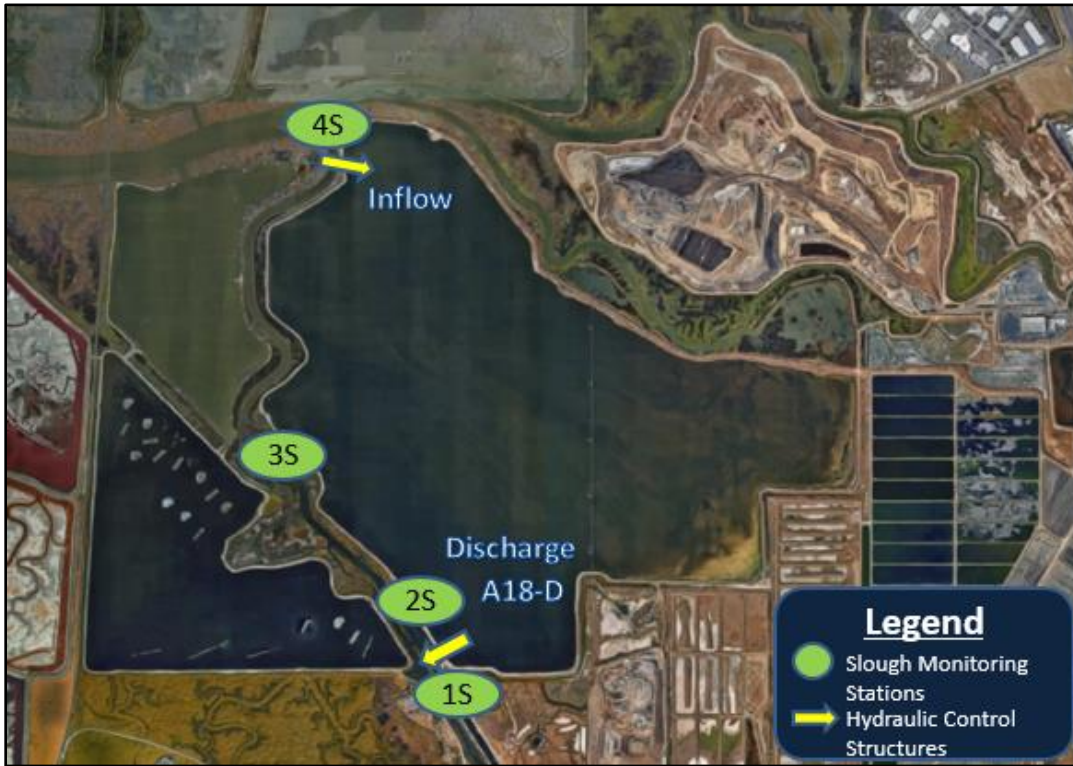
Figure 2. Pond A18 monitoring stations and hydraulic control structures- Southern Discharge. Arrows indicate the flow of water through the control structures.
