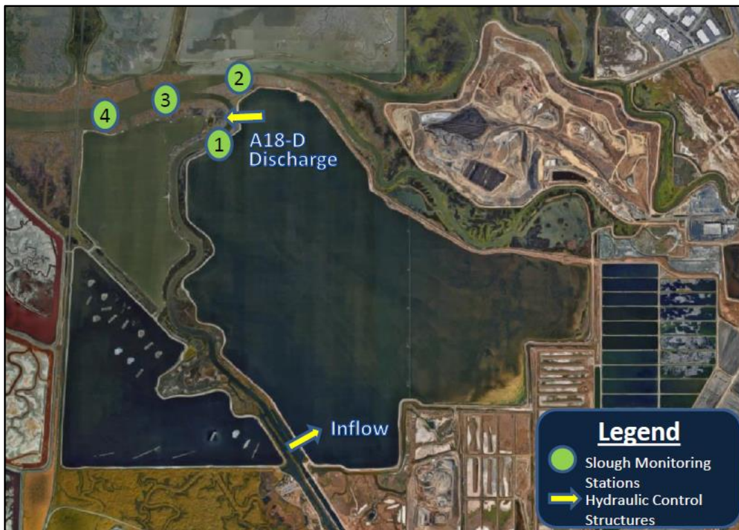
Figure 1. Pond A18 monitoring stations and hydraulic control structures- Northern Discharge. Arrows indicate the flow of water through the control structures.
