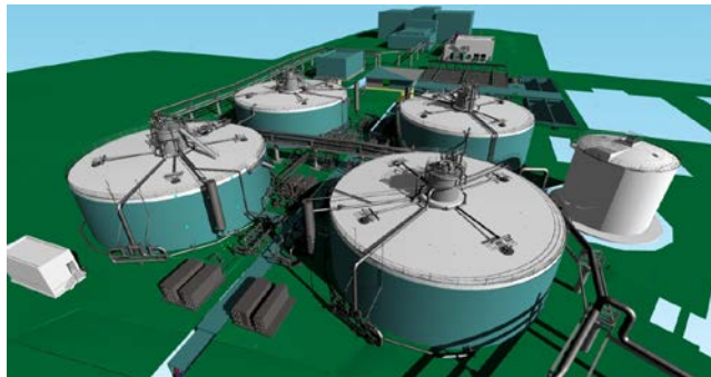
3-D rendering of rehabilitated digesters
