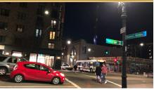
Pedestrian scale lighting illuminates the sidewalk rather than the roadway, providing a more comfortable environment and better visibility at night.
