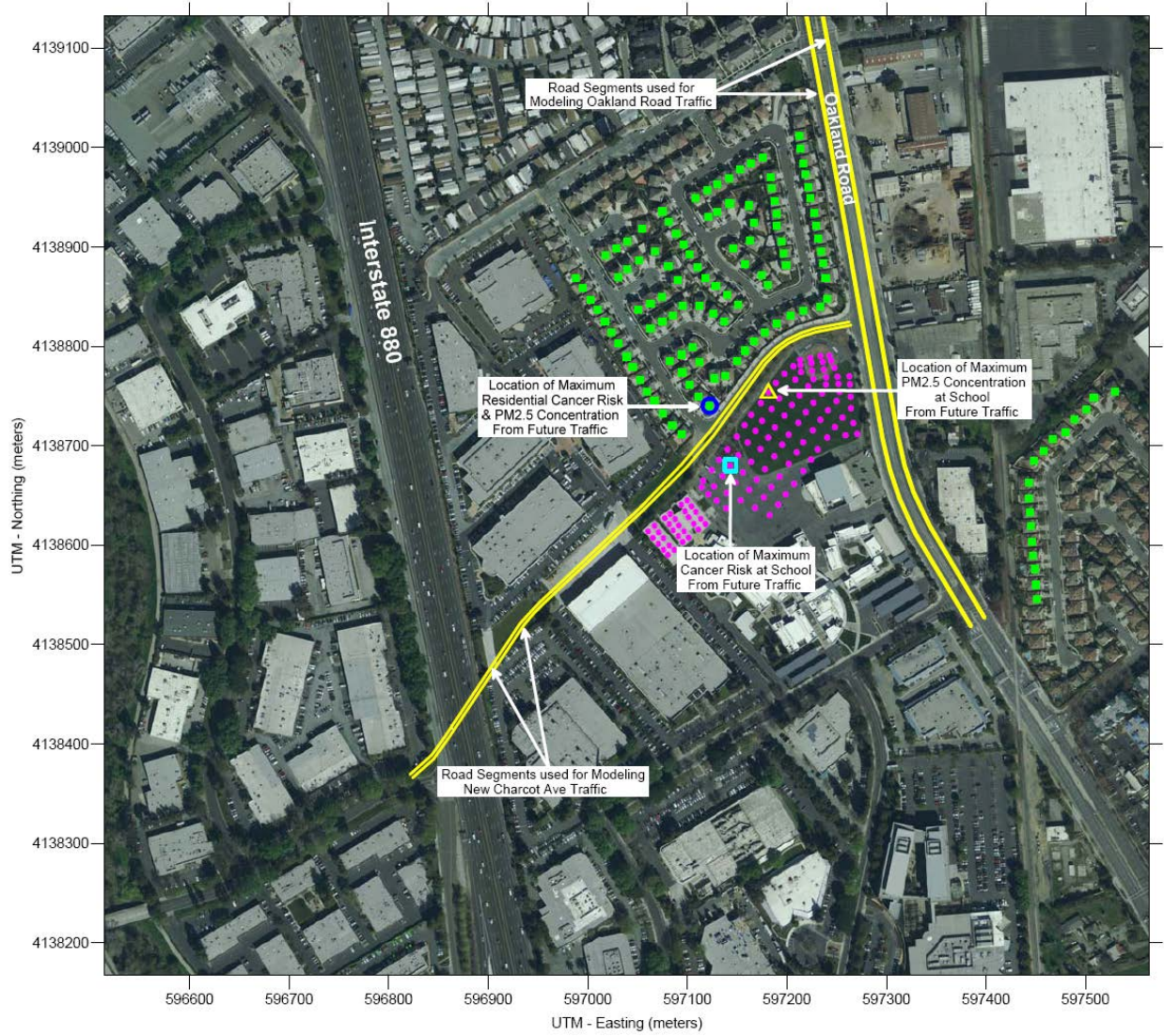
Figure 3. Maximum Impacts from Combined Construction and Project Traffic on Charcot Avenue and Oakland Road Segments
