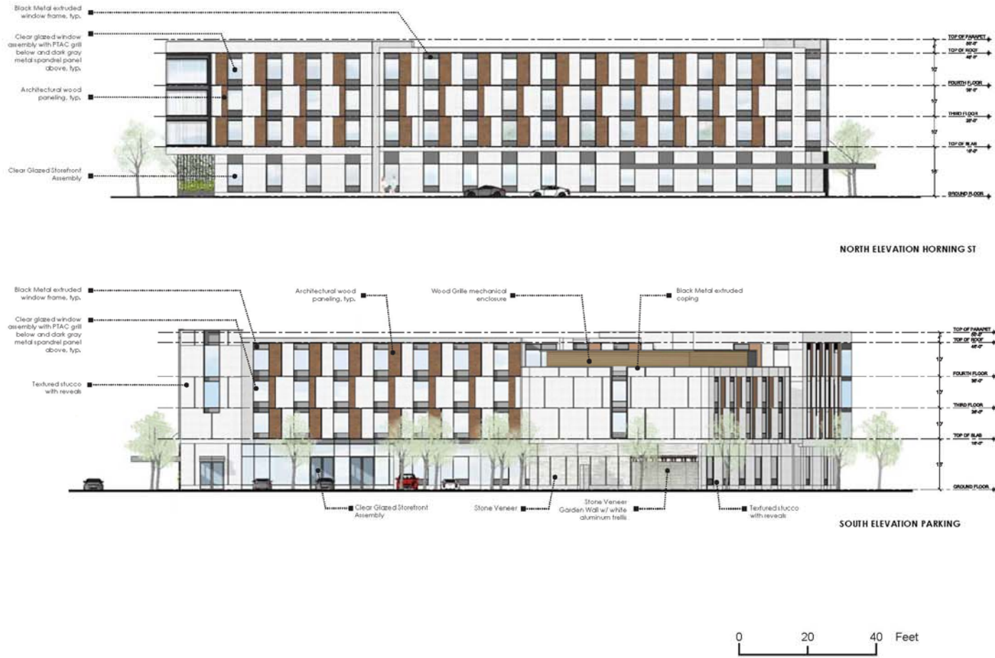
Figure 7 Hotel Elevations (North and South)
